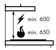
**IMPORTANT** These dimensions are a guide only. All measurements are in millimetres (mm). For complete installation instructions, refer to the manual provided with product.
